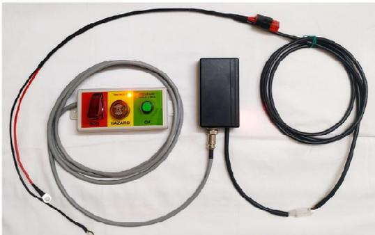
A minimum of 100mm of Track Race Power Supply Cable and Console cable should be left at the unit mounting location for connection to the unit.
